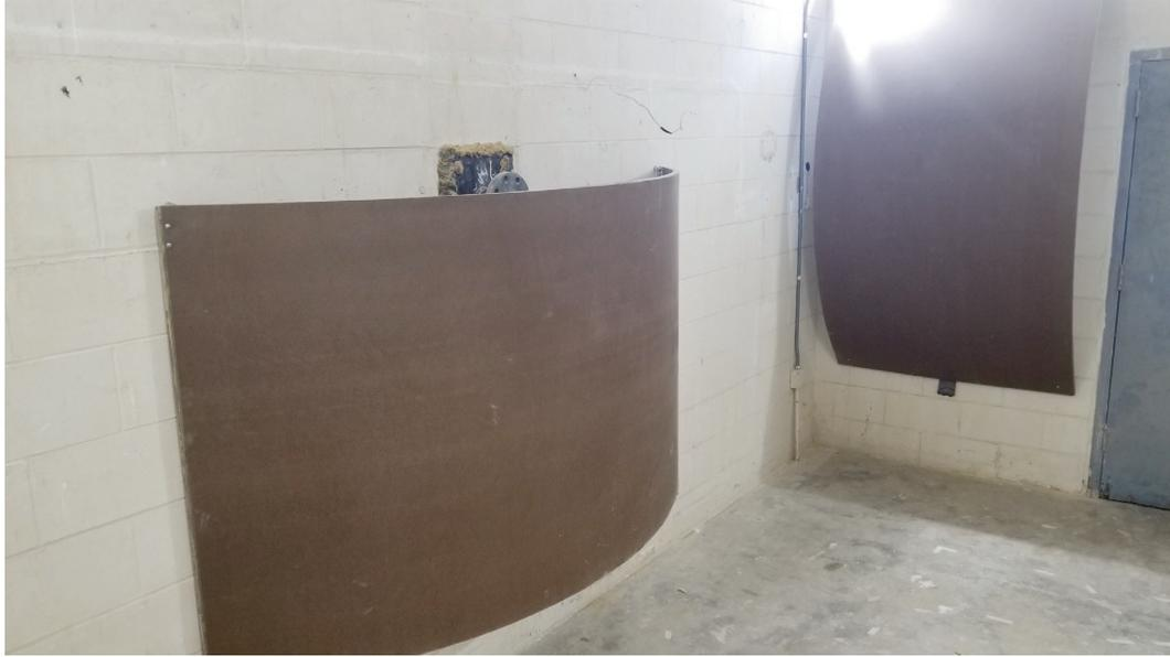
Figure 1-4 Diffusers used for IIC test receiving rooms (an example) reprinted with the permission of Eric Wolfram, see Appendix B.3
