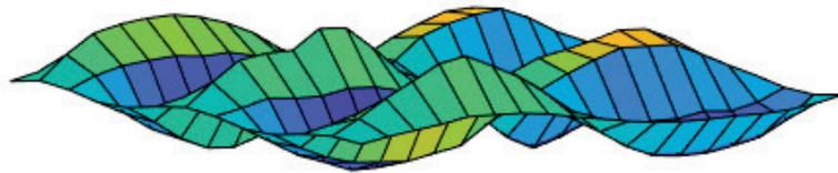
Figure 3-20 Mode shape comparison - 259.7 Hz
