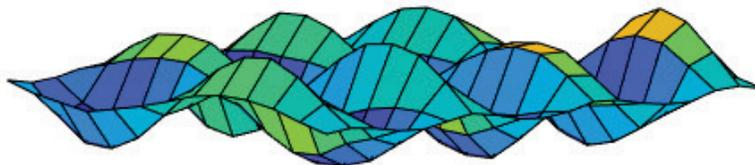
Figure 3-17 Mode shape comparison - 230.9 Hz
