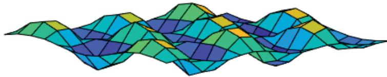
Figure 3-16 Mode shape comparison - 228.9 Hz
